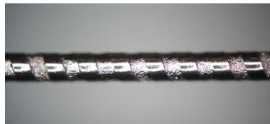
Figure 9. Solder Column Wire after Wave Solder
