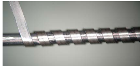
Figure 8. Solder Column Wrapping Process
